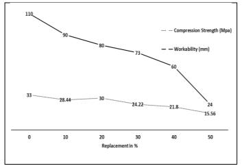
**Chart- 2:** Variation of compressive strength and workability of concrete with replacement of M-sand with laterite residue
