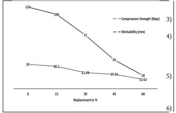
**Chart- 3:** Variation of compressive strength and workability of concrete with replacement of conventional coarse aggregates with crushed Mangalore tiles
