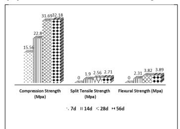
Chart- 4: Mechanical Properties of Optimum Mix Specimens
