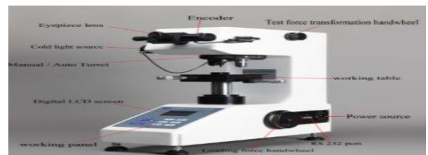
Figure 2: Vickers Hardness Testing Machine
