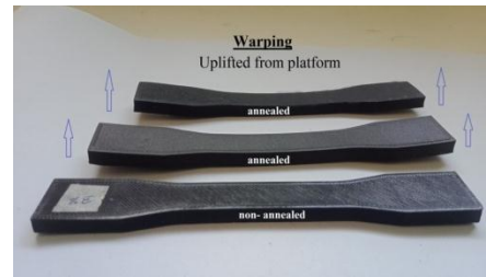
Fig. 7. Warping of 3D prints
