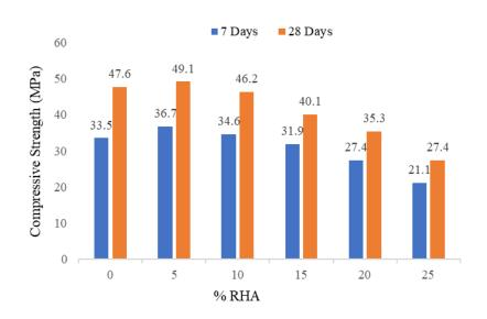
Fig. 1 Compressive strength test results [60]
