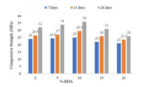
**Fig. 3** Compressive strength test results at 7,14 and 28 days [62]
