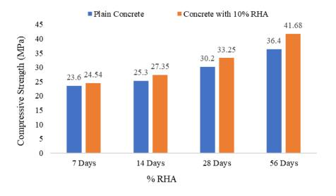
Fig. 2 Compressive strength test results of Plain concrete and 10% RHA [61]
