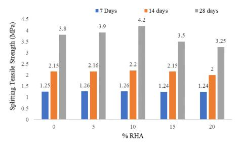
Fig. 6 Split tensile strength at 7,14 and 28 days [62]
