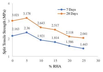
Fig. 4 Split tensile strength [60]
