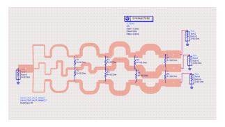
**Fig 3:** Proposed wideband Wilkinson power divider (WPD). Multi section chebyshev matching network
