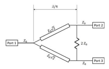
Fig 2(a): Equally-Split 2-way Wilkinson Power Divider
