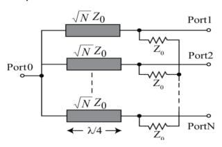
Fig 2(c): N-Way Power Divider for Equal Power Split
