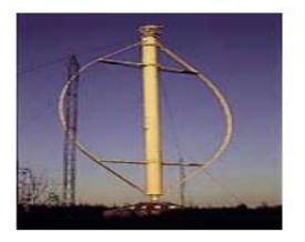
Figure 1.2: Vertical axis wind turbine
