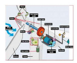
Figure 1.3: Parts of wind turbines
