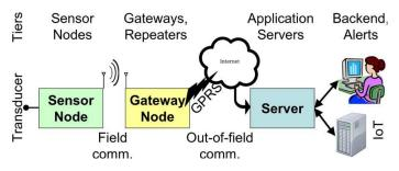
Figure 8 Tiered structure of the WSN platform.
