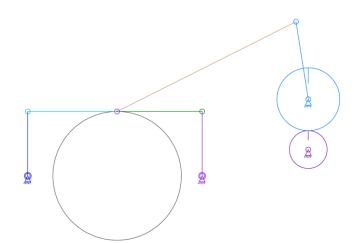
Fig. 6 Eight Link Gear Mechanism in Configuration VI and Possible Coupler Curve
