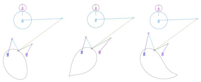
Fig. 1 Eight Link Gear Mechanism in Configuration I and Possible Coupler Curves
