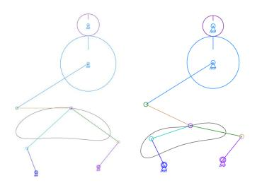
Fig. 2 Eight Link Gear Mechanism in Configuration II and Possible Coupler Curves
