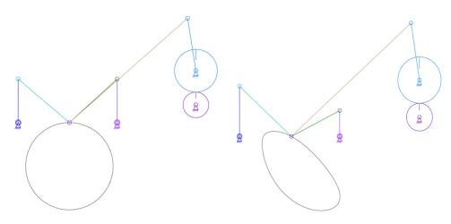
Fig. 4 Eight Link Gear Mechanism in Configuration IV and Possible Coupler Curves
