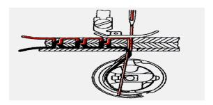
The sewing process is another important one which mainly used the needle descends type of principle. Which is mainly used for tied the flower arrangements it involve looping process to make continuous flower tie arrangement the knot will been varying depend on the flower size .so speed of sewing machine is controlled by servo motor.
