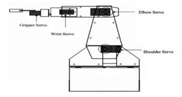
The robotic arm which is very important part in the system it is mainly having different rotation, like positional, linear, and continuous. But our robotic arm we used the positional rotation which is having 180 degree process in motion. It contains four servo motor for four different motions like gripper, wrist, elbow, shoulder function. This operation are done mainly for picking flower IR sensor are used to sense flower position and give the signal to robotic arm to pick and place the flowers.
