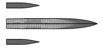
Fig - 4: Configuration of the Trimaran
