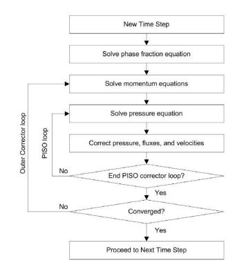
Fig – 5: Flow chart of the pressure evelocity coupling procedure of solver interFoam
