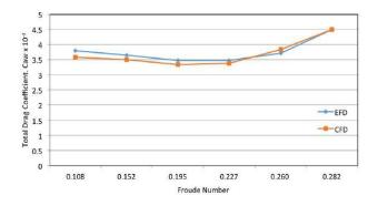
**Fig - 3:** Total drag co-efficient for KCS model at various Froude no., Fn
