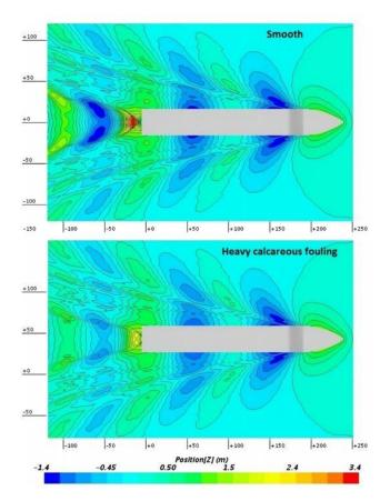
Fig. 6. Wave pattern around the KCS for smooth and heavy calcareous fouling conditions (V= 24 knots).
