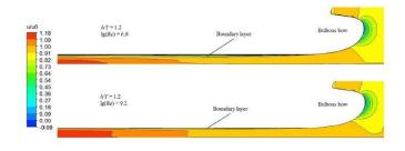
Fig - 2: Contours of velocity at y=0
