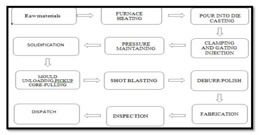
Fig- 3. Process flow of Pressure Die Casting
