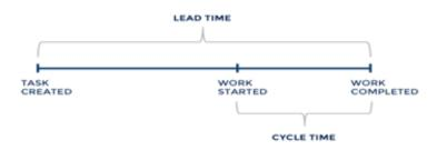
Fig- 4. Lead time and Cycle time
