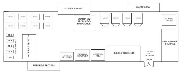
Fig- 2. Optimized Layout of Pressure Die Casting Process
