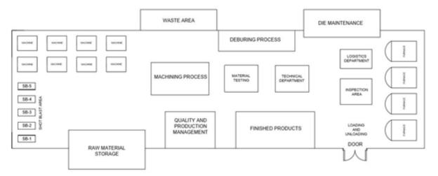
Fig - 1. UnOptimized Layout of Pressure Die Casting Process.
