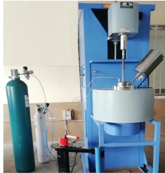
Fig-2: Experimental setup of stir casting process
