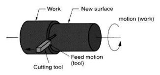
Fig.2. Turning operation [40]
