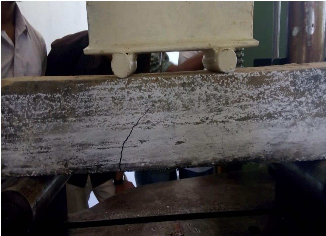
Fig 3.8 Failure of beamspecimen
