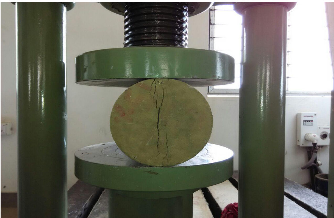
Fig 3.14 Failure of cylinder specimen
