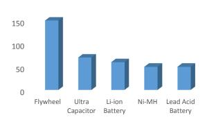
Fig -2: Operating Temperature for Different RBS
