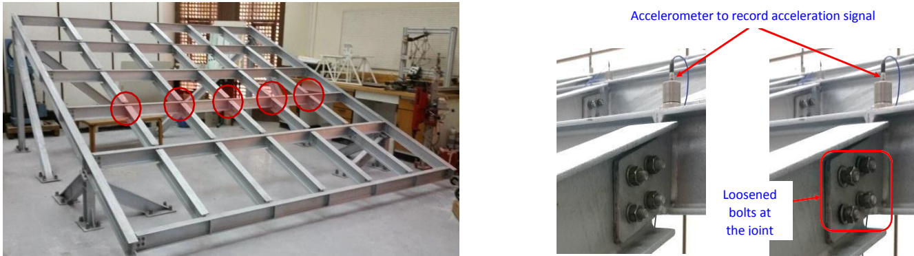
Figure 0.10 The model structure and the accelerometer position, as adapted from [44]
