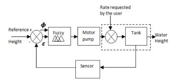
Fig -3: Block Diagram for monitoring system using Fuzzy Logic
