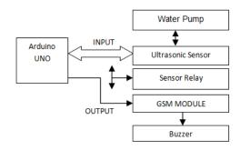
Fig -2: Block Diagram for monitoring system using GSM model
