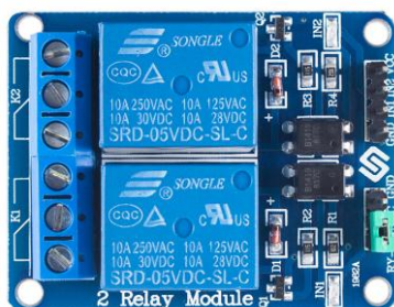
Fig 7: 2- WAY RELAY MODULE
