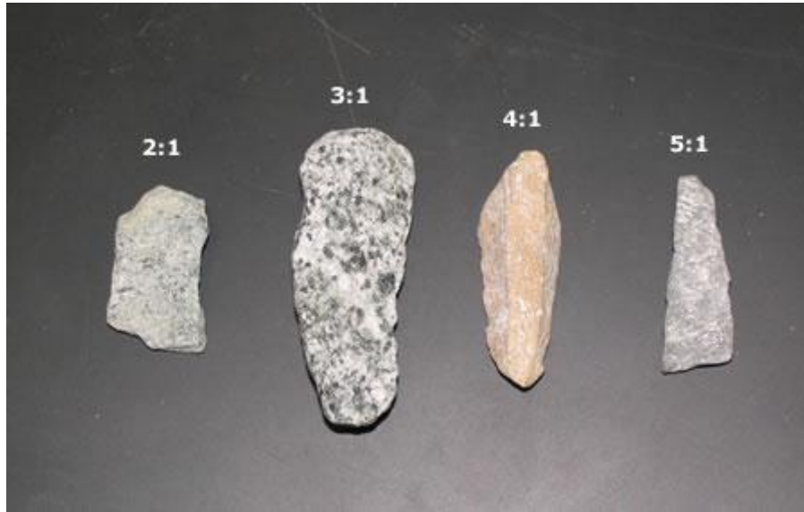
Figure 6 Range of flat and elongated particle ratios. The 5:1 particle is very flat, giving a length: height ratio of 5:1. The height: width dimensions seen in the photo are about 4:1.
