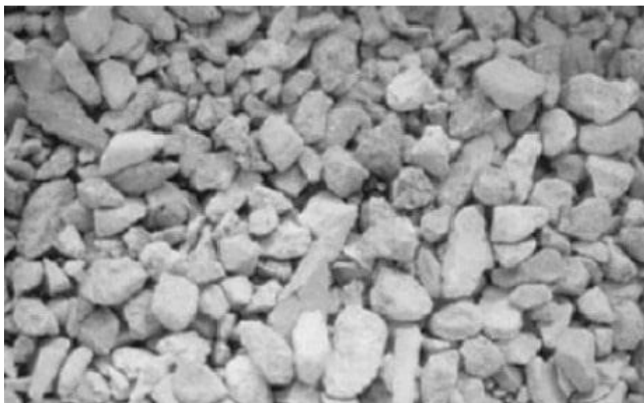
Fig.3. Recycled Aggregates from Masonry Construction Demolition
