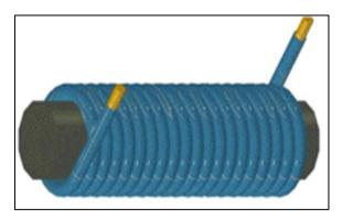
Figure 5. Electromagnet
