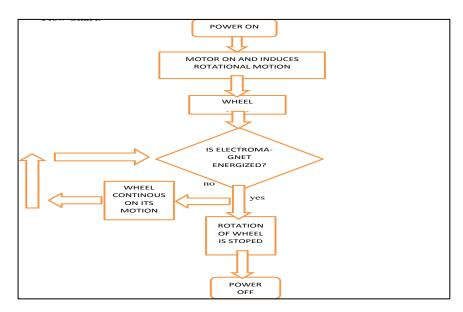
Figure 1. Flow Chart for Working of Electro Magnetic Brakes
