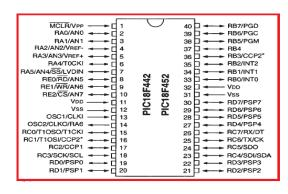
Fig -1: Pin Diagram of PIC 18
