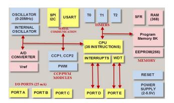
Fig -2: Architecture of PIC18
