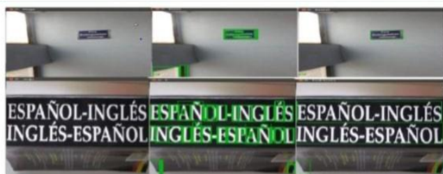
Fig 4.2: Text Detection using MSER algorithm on image captured by mobile camera (top row) and ICDAR 2011 dataset image (bottom row). (a) Original Image (b) Detected MSER Regions (c) Text Regions obtained after applying proposed algorithm
