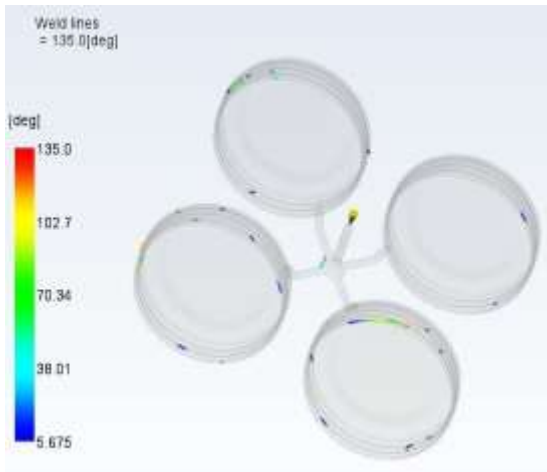
Fig. 7G) Weld line analysis result
