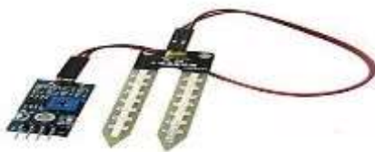
Fig -4: Moisture Sensor
