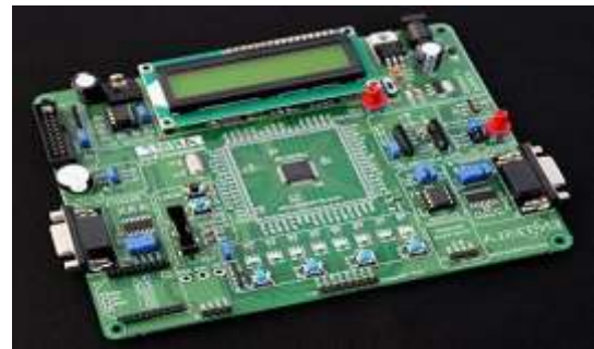
Fig -5: ARM Processor
