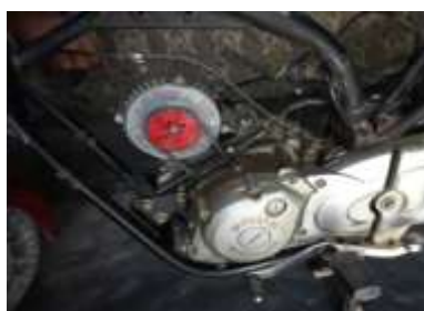
Fig:11 DC Motor fixed with engine
