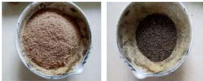
Fig -6: Biomass and bio-char after the pyrolysis
