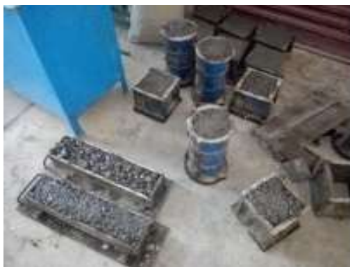
Figure 2 Casting of specimens
