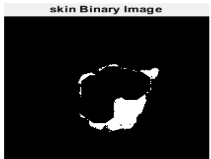
Fig - 1(g): This identifies true skin pixels using the probability threshold which is approximate to 1.
