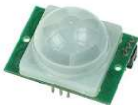
Fig -2: PIR Sensor model diagram
