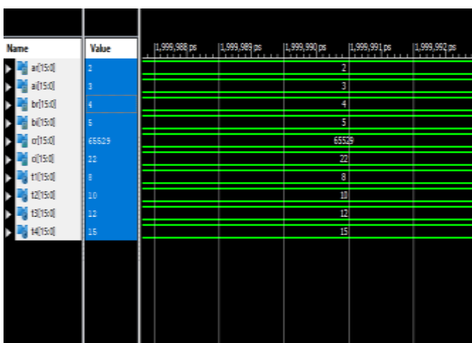
Fig -11: Simulation output for DA based complex multiplier(unsigned number)
