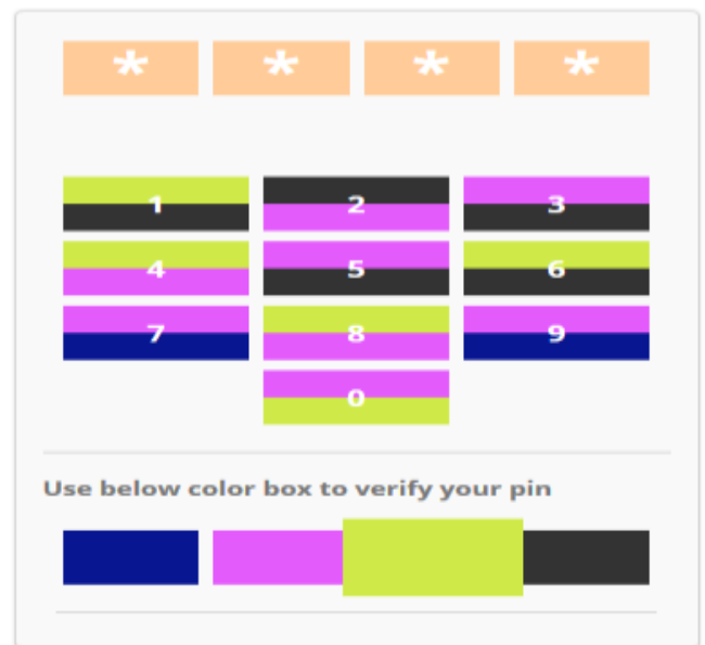
Fig 4: color palette implementation: user selects the green color for first pin number 1 to validate it.
