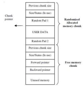
Figure 6: Allocated heap memory chunk with dual random padding [20]
