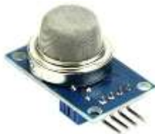
Fig -4 Gas Sensors(MQ6)
