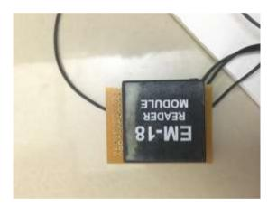
In addition, when an ambulance is approaching the junction, the RFID reader placed in each signal reads the vehicle with the tag and it will communicate to the traffic controller in the junction to turn ON the green light until the ambulance passes and the red light for the other path should be turned red.
