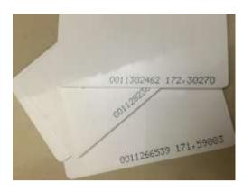
Each individual vehicle is equipped with special radio frequency identification (RFID) tag which is placed at a specific location which cannot be removed easily. If the RFID-tag-read belongs to the stolen vehicle, the location is tracked using GPS and then a message is sent using GSM to the police control room.
