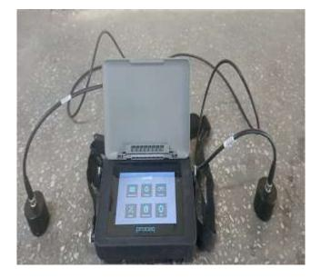
Fig- 1: Ultrasonic Pulse Velocity Test Equipment (Proceq Model- PL 200)
