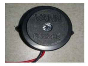
A buzzer is a device that produces sound. The working principle of the buzzer is mainly based on the theory that, whenever an electric voltage is applied across a piezoelectric material, a pressure is generated. A Piezo buzzer contains
