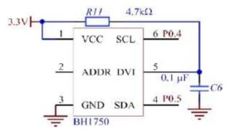
Fig-4: Pin diagram of BH1750
