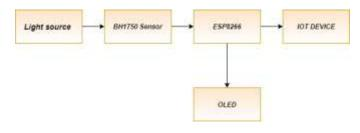
Fig -5: Block diagram of the System
