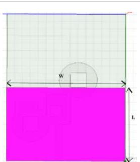
Fig 2: Bottom view of the patch antenna
