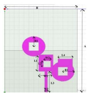
Fig 1: Top view of the patch antenna
