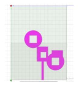
Fig 4: Actual design of the patch antenna
