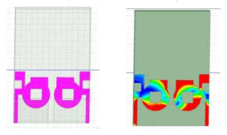
Fig 6:Two patch antennas of same sructure (TPASS). Fig 7:Electric Feild distribution of the anenna.
