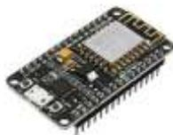
It is an open-source firmware and development kit that helps you to prototype or build IoT product. It includes firmware which runs on the ESP8266 Wi-Fi SoC from Espressif Systems, and hardware which is based on the ESP-12 module. The firmware **uses** the Lua scripting language
