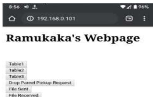
So for controlling purpose we use webserver. By which we can access and control bot. We are using webserver which is generated by node MCU itself. We design webserver as per our requirement. We created buttons which actually call the bot from table to table whenever we required. We also add file acknowledgement system that is whenever bot come at the
