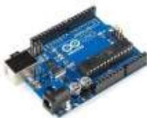
The Arduino Uno is a microcontroller board based on the ATmega328. It has 20 digital input/output pins (of which 6 can be used as PWM outputs and 6 can be used as analog inputs), a 16 MHz resonator, a USB connection, a power jack, an in-circuit system programming (ICSP) header, and a reset button.
