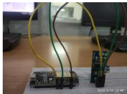
Fig-8: Connection diagram for interfacing flame sensor with Node MCU.
