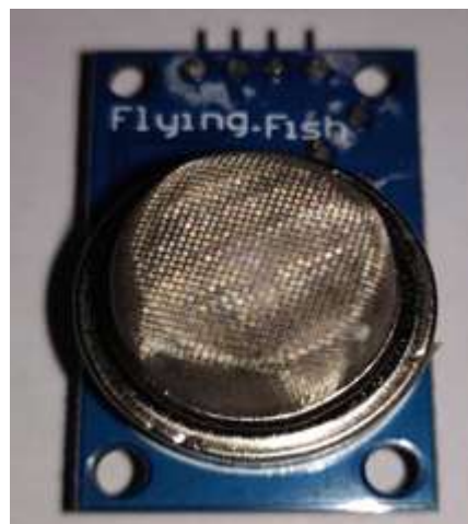
Fig-4: Gas Sensor
