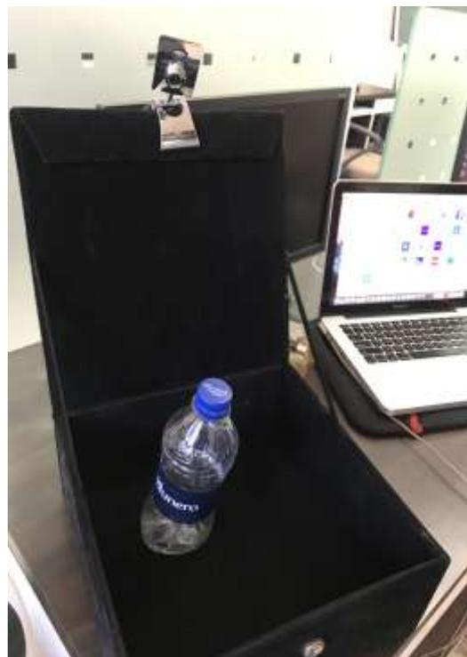
The above figure is the system in which it consists of a box in which camera is mounted on a top when object is placed in the box camera detected an object.
