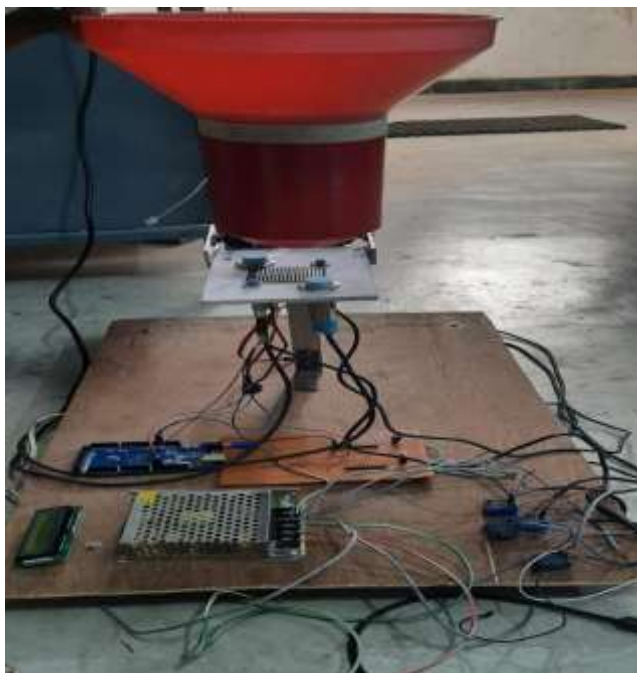
Fig - 4: Automated Waste Segregator System
