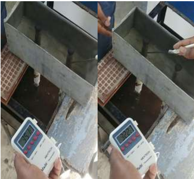
Fig. 6 And the heat pipes difference of temperatures with wick (35 o c) and without wick (32 o c) materials
