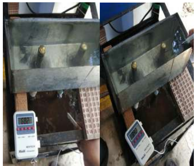
Fig. 5 Arrangement of heat pipes with source tank includes heater and sink tank to measure the temperature readings
