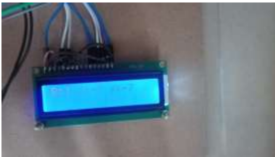
LCD displays the Accelerometer sensor Values(x,y)
