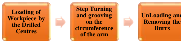
Figure 11 FLOW CHART OF TURNING PROCESS
