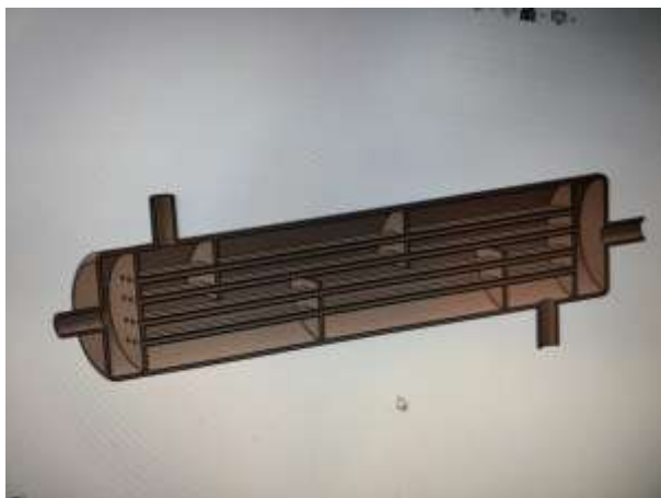
Fig 7: Heat Exchanger with 4 baffles
