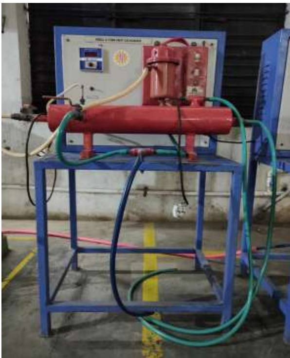
Fig 4: Experimental Setup of Shell and Tube Heat Exchanger
