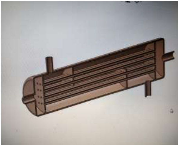
Fig 6: Heat Exchanger with 2 baffles
