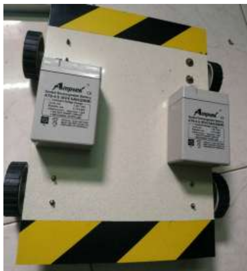
Fig. Power supply to the robot using batteries
