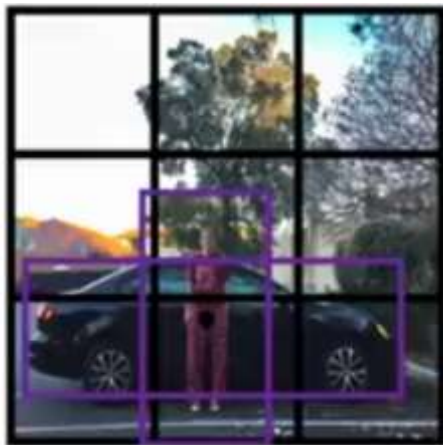
Fig. 2- Detection of object using anchor box
