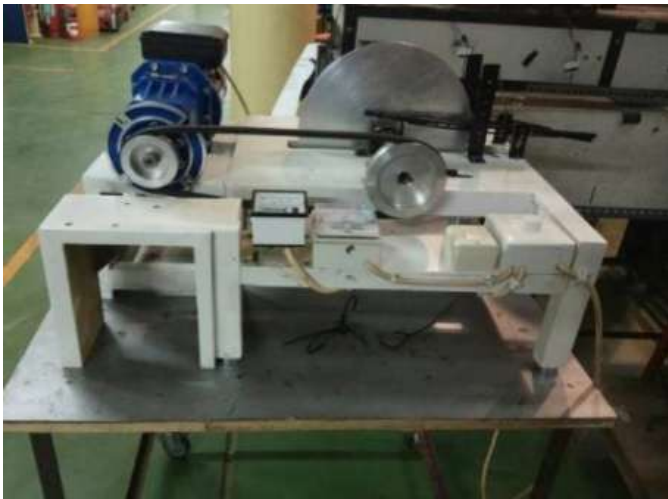
Fig.6- Disc Type Oil Skimmer
