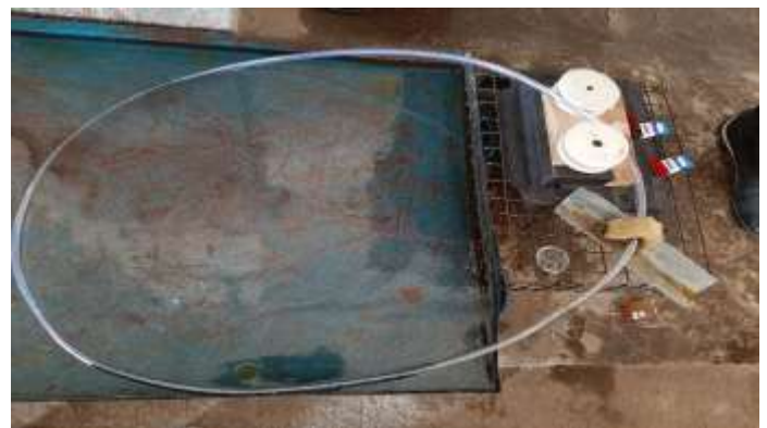
Fig.7- Pipe Type Oil Skimmer
